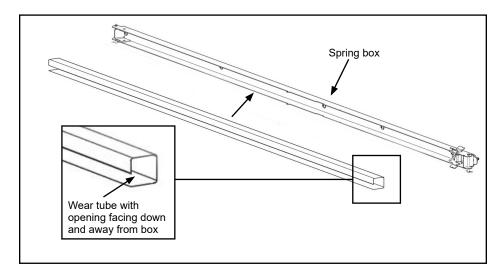
B. Place spring inside of wear tube (not shown below for illustration purposes) on ledge of spring box with spring loop on opposite end of pulley bracket. Push bushing into spring loop and align with holes in spring box. Insert 3/8" x 2-3/4" bolt into bushing, secure with nylock hex nut, tighten until snug.
