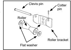
B. Position roller guide 1/4" from latch plate. Lowest point of roller should be flush with or slightly above top surface of box.
