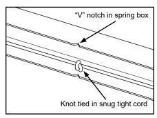
C. Pull cord through pulley bracket, stretching spring and place knot in pulley bracket slot.
