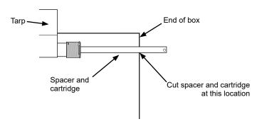
B. Measure in 1/2" from cut end and drill pilot hole, then drill 5/16" hole through spacer and cartridge.
