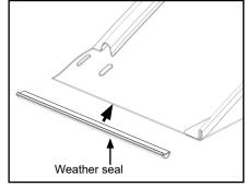
D. Peel protective backing then adhere seals to each side of end cap.
