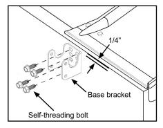
C. Place remaining base brackets 1/4" down from top of box, drill (2) 5/16" holes and secure with 3/8" x 1" self-threading bolts.
