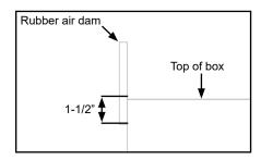
B. Use pre-drilled holes in rubber as guide to drill 7/16" holes. Install 3/8" x 2" bolts with fender washers on the outside of rubber. Secure with flat washers, lock washers and nuts on inside of box.
