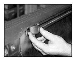
B. Slide carriage bolt bracket and 5/16" x 1-1/4" carriage bolt into channel of Deck Rail System, one set per side rail bracket.
