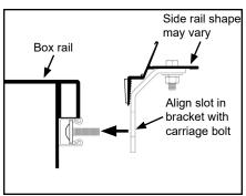
E. Secure with 5/16" serrated nut. Leave finger tight for now.
