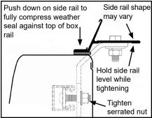
G. At front bracket, ensure side rail is parallel with box rails, then torque serrated nut on front bracket to 20 ft-lbs.
