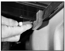
F. At marked locations drill 1/8" holes through box rails, then attach header bar to box rails with (4) 1" self-threading hex bolts; do not tighten yet.
