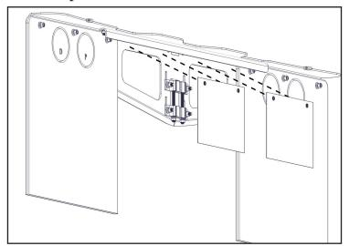
3. Peel protective layer off adhesive pads. Do not touch adhesive with finger. Adhere pad to back of frame as shown in Figure 3. Press pad firmly onto mud flap frame.
