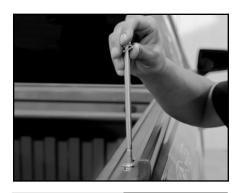
D. Remove rear taillight assembly and place clamp plate underneath stake pocket.
