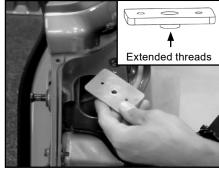
E. Thread long bolt into clamp plate.
