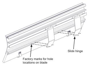
F. Insert (2) square nuts with flat side facing up in top channel of blade end and align with slide hinge top holes.
