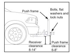
**NOTE:** In some cases, clearance under receiver may be less than 6". If so, plow will still operate properly, but ground clearance will be limited. Use care on uneven surfaces.
