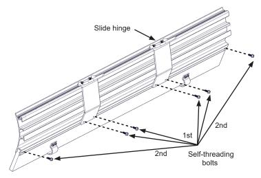
L. Hang 1 end of blade assembly into closest retainer groove on push frame. Repeat for opposite end of blade assembly.
