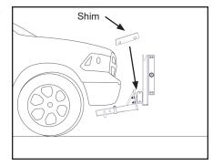
G. If push frame leans away from front of vehicle, remove lower bolts and insert one or two shims at bottom as shown and reinsert bolts.
