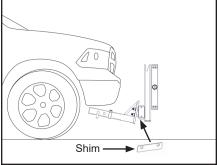
H. Secure (4) 1/2" x 4" bolts with (8) flat washers and (4) lock nuts. Torque 4 nuts to 90 ft-lbs.
