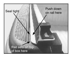
D. Start at front of box. Install 1st clamp 1-1/2" from inside of box.
