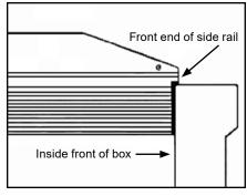
B. At front, adjust top of side rail flush with top of box. Then secure front of side rail to box with locking pliers. See locking pliers at front in illustration on page 3.
