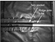
C. Insert front and rear tube extensions into ridge pole.
