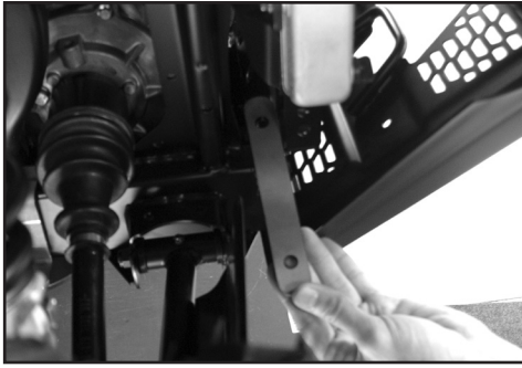
G. At front of machine, place front bracket on top of machine frame behind front shield.
