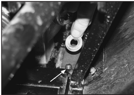
K. From top, add flat washer and start lock nut on bolt. Repeat on bolt hidden from view on opposite side.
