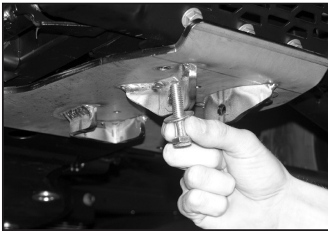
J. From under machine insert a long bolt (2) with washer into front hole. Bolt goes through plate, through hole on machine and into hole on front bracket (hidden from view).
