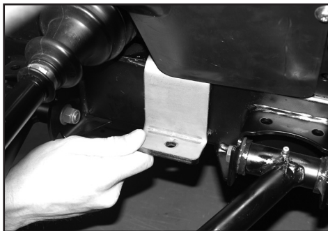
B. View showing right rear mounting bracket in place. (tab behind gusset, hidden by wheel well shield in photo)
