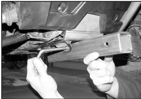
N. Lift front of receiver up and insert hitch pin through holes on mount plate and through receiver to opposite side.
