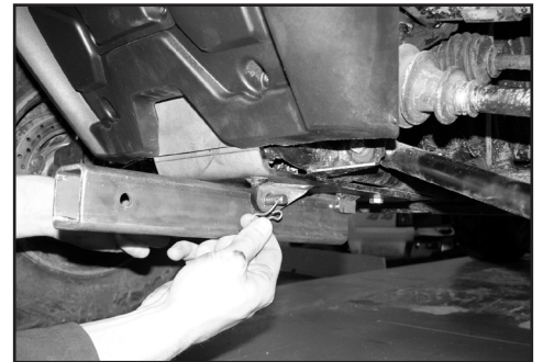
O. Insert hitch pin clip. Installation is complete. Periodically check torque on bolts and retighten if needed.
