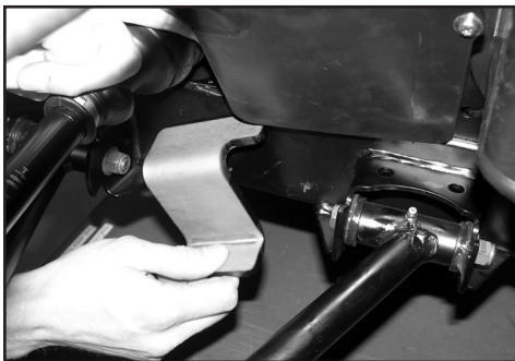
A. Right side: From behind front shaft, place right rear mounting bracket along side of machine frame. Orientate bracket so tab rests along side of gusset and on top of frame.
