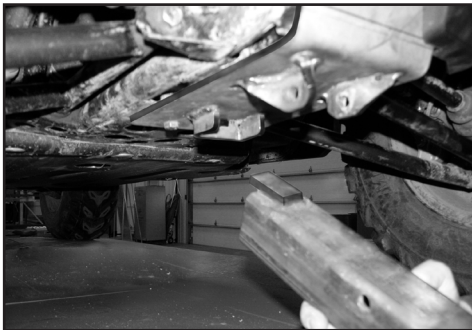
M. Insert prong of receiver into notch under rear of mount plate.
