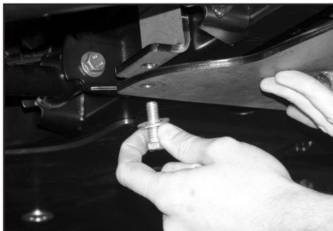
E. From under machine, lift mount plate up as shown, hold it and insert a short bolt (2) with washer through mount plate and rear bracket directly above (both sides). Turn each lock nut tight enough to hold mount plate up but do not fully tighten yet.
