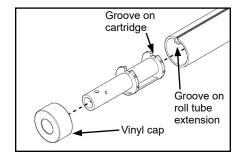
B. Measure 6-1/2" in from beginning of drive cartridge and 180° opposite of rope channel and mark.
