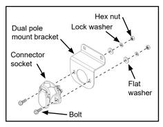
B. Before cutting wire, form a loop on arm that allows room for movement and mark where to cut at connector socket at location on dual pole mount bracket. Cut wire, strip only enough insulation off to attach ring terminals and heat shrink tube. Attach wires to socket terminals.
