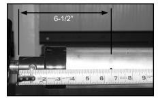
C. Drill 5/16" hole through first wall of roll tube cartridge.
