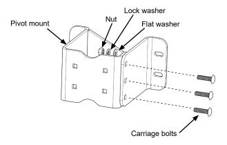
B. Slide (4) square nuts into channels in mounting plate. Secure pivot mount to mounting plate using (4) 3/8" x 1" stainless steel bolts, flat washers and lock washers threaded into square nuts in channel. Center pivot mount on mounting plate and finger tighten all hardware.
