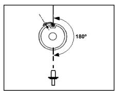
D. Insert 5/16" x 9/32" drive rivet. Ensure rivet is fully seated. Set with hammer.
