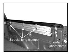
B. At front, position clamp next to header bar and as far forward as possible, or if no header cross bar, near end of cargo rail.
