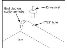
C. Pull tarp by hand to stretch tight along stationary tube. Drill 7/32" hole and insert drive rivet. Ensure it is fully seated and set with hammer.
