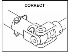
F. Ensure U-joint is in correct position for maximum strength when locked at 90° angle. Make correction if needed.
