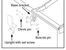
**NOTE:** If installing rubber uprights, drill 5/16" hole through rubber in line with stationary tube at front and rear. Start 3/8" x 1-1/4" self-threading bolt, bolt will be tightened in Step 13.
