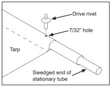
D. Cut stationary tube 1/4" beyond edge of tarp. Grind smooth, then install end plug.
