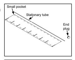
B. Extend stationary tube 1/4" beyond edge of tarp. Drill 7/32" hole and insert drive rivet. Ensure it is fully seated and set with hammer.
