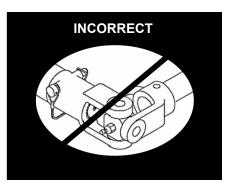
G. Ensure lock pin is in correct position around spline shaft. Make correction if needed
