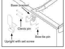
**NOTE:** If installing rubber uprights, drill 5/16" hole through rubber in line with stationary tube at front and rear. Secure with 3/8" x 1-1/4" self-threading bolt.
