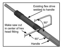
B. Grind weld and fitting flush with handle until new flex drive slides fully onto handle.
