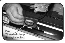
A. Orientate clamp plate on cord assembly to drop welded side down through slot in rail so it falls into stake pocket. Hold cord while doing this to support clamp and alignment plates throughout the following steps. NOTE: Some stake pockets may be deformed, if so, it may be necessary to grind material off of spacers.
