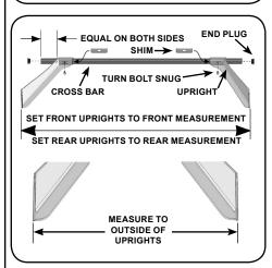
C. Slide front cross bar (the bar without reflective decal) in uprights. Space bottom of uprights to match front measurement taken earlier between rails. Center cross bar. Turn set bolt in temporarily snug enough to prevent cross bar slippage. Tap end plug into each end of cross bar.
