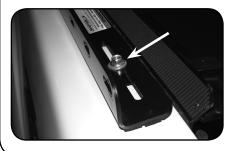
E. Slowly close tailgate to make sure it will not rub against rack rail when closed. (Adjust rack rail forward if needed). Now fully tighten all clamp bolts. Repeat for rack rail on passenger side of box.
