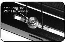
D. Place flat washer over hole and thread a hex head bolt into threaded clamp inside stake pocket. Turn until finger tight. Ensure that alignment plates are aligned with stake pocket. Then remove cord. Repeat A through D for all remaining stake pockets.
