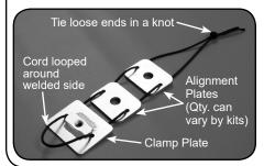
A. Assemble all threaded clamps and alignment plates to cords as shown. First, loop cord around clamp plate so welded side with threaded hole is at bottom when lifting cord up. Then add all alignment plates equally. When done, each cord should have a threaded clamp plate with equal amount of alignment plates. Tie knot at top of cord.
