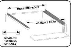
A. Measure distance between inside rails at selected front location.
