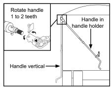
**NOTE:** To adjust tension, unroll tarp and remove all tension. Rotate handle 1 to 2 teeth, reassemble and check tension. Repeat until proper tension is achieved.
