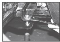
b) Draw bolts tight evenly on each side-9/16" wrench. **Torque bolts to 31ft.lbs.**
