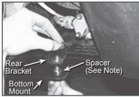
a) For machines without skid plate, from bottom insert bolt up through mount plate, then 1 spacer, then through bracket. From top lay flat washer over bolt and turn lock nut on finger tight only.
