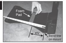
a) For ATV's without skid plate, measure back 4 ½" on plow mount plate as shown. Wipe area clean and make mark. Apply adhesive side of foam pad next to mark as shown. NOTE: If ATV has a skid plate, foam pad is not used. Leave skid plate on and start with b) at right.
