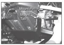
b) At front of machine, position and support mount plate up under frame with tabs to front of differential. Insert mount pin through hole in tab-then direct pin over top of machines frame, push it all the way through and into hole in tab on opposite side. (Tires may need to be turned)
