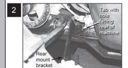
a) Orientate rear mount bracket behind front tire/axle area as shown. View is of left side of machine. Note direction of flange legs with hole toward rear of machine.
