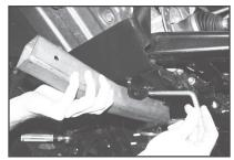
b) Lift front of receiver up and insert receiver pin through flange mount plate, receiver and flange on other side.
