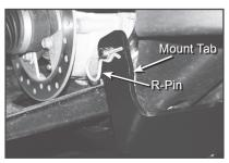
c) At other side, push R-Pin into hole on mount pin. Mount can hang from frame for now.
