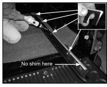
C. Set entire assembly back on box. Align holes to reuse original 10 mm bolts. Press down on box rail at rear to make double sided tape reattach to truck body.
