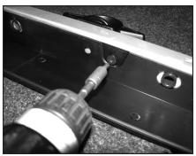
D. Position side rail in between utility rail and box rail.
