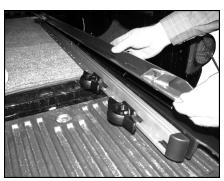
E. Insert a shim at each 10 mm bolt location, excluding the one at rear. See Step 3A and 3B for positioning and quantity of shims.
