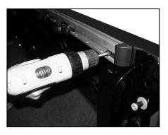
B. Use 10 mm socket with ratchet to remove hex bolt at front corner of box. Save for later.
