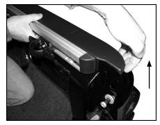
C. Use T-25 wrench/driver to remove Torx bolts (star head) holding box rail protector to utility rail and replace with screws (included in kit). Leave loose for now.
