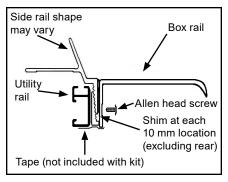
B. Tighten Allen head screws to hold utility rail, shims, side rail and box rail together as an assembly.
