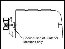
C. At front, insert bolt, lock washer and flat washer through hole in cargo rail, then a clamp half (no spacer) on opposite side and start threads. Repeat at rear of cargo rail.
