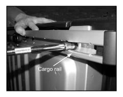
B. Cargo rail is still loosely attached to box with 2 nylon anchors. Starting at front, pull cargo rail until anchors disengage and cargo rail is free from box.
