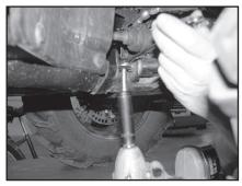
c) Then tighten both rear bolts snug tight. (9/16 size wrenches) Now torque each front bolt to 31 ft. lbs. Then torque each rear bolt to 31 ft. lbs.
