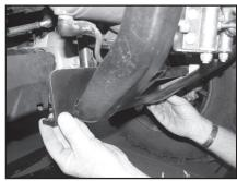
c) When done, bracket should nestle on top of machine frame as shown.
