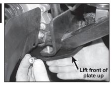
a) At front of machine, lift front of mount plate up and insert short bolt bottom up through mount plate and into hole on front bracket. Then use flat washer and turn lock nut on finger tight. Insert another short bolt, flat washer and finger tight lock nut on opposite side.
