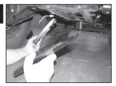
a) Under rear of machine, from side as shown insert rear bracket on mount plate across top of rear frame tubes (and under drive shaft) until open hole in bracket extends on outside of frame on opposite side.
