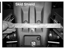
a) Under machine at front, hold straight edge ruler across center of front two bolts on skid shield as shown.
