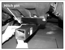
b) Lift front of receiver up and insert receiver pin through receiver and mount plate.
