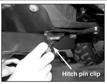
c) Insert hitch pin clip into receiver pin.
