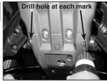
a) Drill 13/32" hole at center of marks through plastic skid shield only. Use care when drilling.
