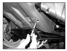
c) Align holes in front of mount plate with holes drilled in skid shield. Insert bolt in each hole through mount plate, skid plate and until threads protrude through mount bracket. (mount bracket is on top of frame behind skid shield hidden from view) See photo 3a for view from top.
