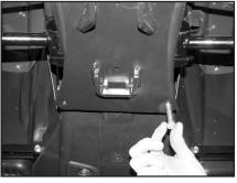
b) Insert a bolt from bottom up through each hole in mount and push it through hole drilled in plastic skid shield.
