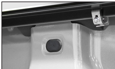
WATER RESISTANT FOAM WEDGES Close gaps under the box rail
