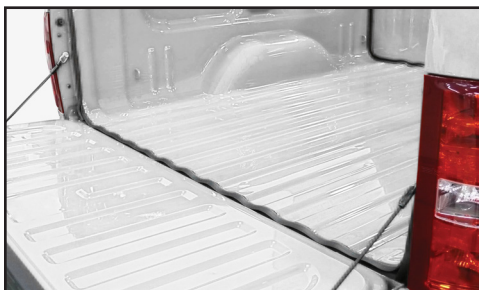
SEALING GASKETS Seal gaps at the front and rear of the box
