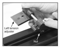
B. Turn 1-1/4" bolt with flat washer onto nut in front bar. Leave loose for now. Repeat for tension adjuster (marked "R") on passenger side of cover and leave bolt loose as well.
