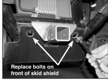
c) Replace 2 original bolts with washers to secure plastic skid shield in place. Installation is now complete. Periodically check bolts and retorque if needed.
