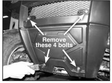
a) At front of machine, remove 4 bolts on shield with T27 torx wrench.
