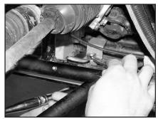
b) Using 9/16 wrenches, hold nut at top and tighten bolt from bottom. Repeat for each bolt.
