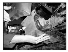
b) Pull bottom of shield away from machine far enough to allow front of mount plate to fit behind shield and up against frame.
