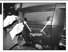
a) At front of machine, insert (2) top bolts (removed earlier) into shield and tighten with T27 torx.
