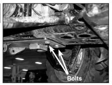
a) Photo shows both bolts in place under back of mount plate ready to be tightened.
