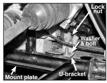
c) Place flat washer over each bolt and turn lock nut onto each.
