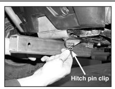
c) Insert hitch pin clip. Installation is complete. Periodically check torque on bolts and retighten if needed.
