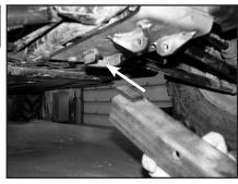
a) Insert prong of receiver into notch under rear of mount plate.
