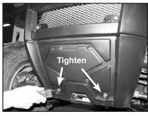
b) Then tighten bottom 2 bolts on shield with T27 torx.
