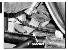
a) Behind front drive train, place U-bracket on top of frame between tubes under cable. (Also see photo 2c at right)
