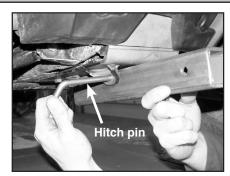
b) Lift front of receiver up and insert hitch pin through holes on mount plate and through receiver to opposite side.
