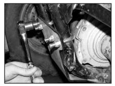
c) At front of machine tighten and torque nuts on each U-bolt to 31 ft. lbs.
