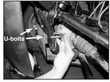
c) Support mount plate up in position. Install U-bolts from behind around frame tube and into holes of mount plate. Turn lock nuts on both Ubolts.
