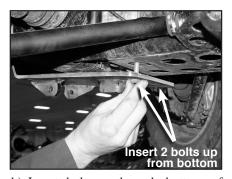
b) Insert bolt up through bottom of mount plate and through hole in Ubracket (2 bolts).
