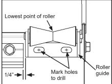
D. Drill (2) 5/16" holes at marks. Secure bracket to box with 3/8" x 1" self-threading bolts.
