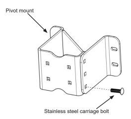
B. Slide (4) stainless steel square nuts into channels in mounting plate. Secure pivot mount to mounting plate using 3/8" x 1" stainless steel bolts, flat washers and lock washers threaded into square nuts in channel. Center pivot mount on mounting plate and finger tighten all hardware.
