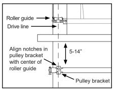
C. Select solid bolting locations (such as rivet lines or ribs) for (2) bolts near pulley bracket (4" and 12" from edge of spring box) and last bolt near opposite end of spring box. Remove knockouts and mark locations.
