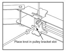
D. Check spring tension after the first open and close cycle of the tarp. Spring is properly tensioned when pulley settles back and lines up approximately with rectangular notch on spring box.
