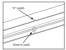
C. Pull cord through pulley bracket, stretching spring and place knot in pulley bracket slot.
