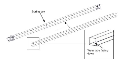
B. Place spring inside of wear tube (not shown below for illustration purposes) on ledge of spring box with spring loop on opposite end of pulley bracket. Push bushing into spring loop and align with holes in spring box. Insert 3/8" x 2-3/4" bolt into bushing, secure with nylock hex nut, then tighten.
