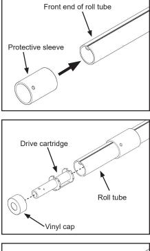
B. Insert drive cartridge into end of roll tube.
