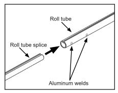
C. Insert second roll tube onto opposite end of roll tube splice until tubes are tight against each other.
