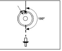
G. Then insert drive rivet. Ensure drive rivet is fully seated and set with hammer.
