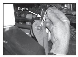
c) Insert R-pin on opposite side to secure mount. **Installation is complete.**
