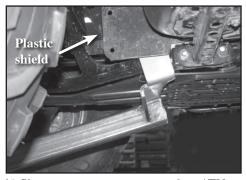
b) Shows mount prongs engaged on ATV frame. Note: When inserted properly, plow mount prong on each side is behind plastic shield. Make sure mount is pushed firmly against machine frame - prongs fully engaged in frame.
