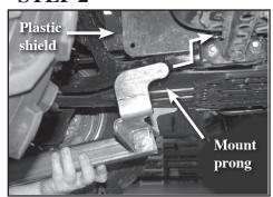
a) Under ATV frame, insert prongs on rear of mount up onto ATV frame behind plastic shield (one prong on each side) and push toward rear as shown.
