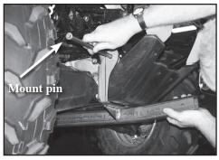
b) Align holes on plow mount with holes on bracket. Insert long pin all the way through both holes on each side of mount.
