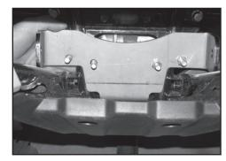
b) Insert U-bolts from behind over tubular frame and into holes on bracket and start lock nuts.
