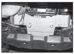
c) Begin drawing both lock nuts snug tight evenly on each U-bolt. **Then torque U-bolts to 10 ft. lbs. (Avoid over tightening).** Turn front wheels to sharp right position.
