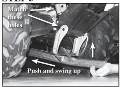
a) With rear prongs of plow mount engaged under machine frame (as shown in step 2-b), lift and swing front of mount up until holes can be aligned with bracket on machine.
