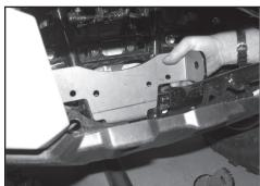
a) At front of machine insert mounting bracket through opening at top of skid plate and wiggle into place until bottom bracket tab slips down and bracket rests on frame.
