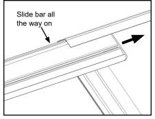
C. Pull vinyl tight (it should stretch an additional 1/2"), then center bar and reinsert Phillips screws (1 at each end, removed in Step 1G) back in their original holes. Vinyl should be tight from side to side (no wrinkles) and extend equally at both ends of bar. If needed, make adjustments.
