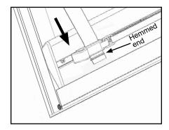
Alternate Method: If vinyl straps were bolted on, reinstall by noting previous mounting locations, cutting a small "X" in each vinyl strap (just enough to allow bolt or screw through) and mount with existing bolts or new screws (screws not included).
