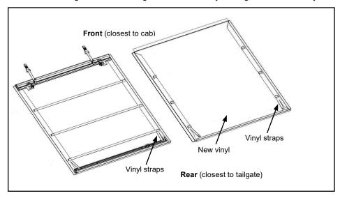
G. At each end of front bar, remove and save Phillips screws. These screws hold the vinyl tight after assembly.
