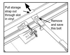
**Snap on:** Pull each storage strap up until free from bar, then pull through slot in vinyl. Save straps for later.
