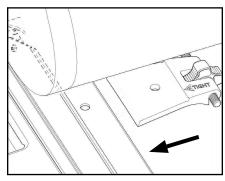
K. Align holes and insert bolt from top, secure with washer and nut. Repeat for tension adjuster on other side. Center bar between side rails.
