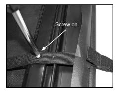
E. Note how vinyl straps attach to rear bar then detach them. Vinyl straps are bolted to rear bar or slide through slots in Slide Locks or latches.
