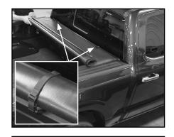
B. At front corner, remove bolt mounting tension adjuster to side rail. Save bolt, nut and washer.
