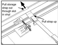
**Screw on:** Remove screw on each storage strap, then pull through slot in vinyl. Save screws and straps for later.
