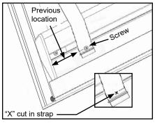
H. Bows are removed by peeling apart hook and loop at both ends of bows. Remove one bow at a time from old vinyl and install in same position on new vinyl. When done, inspect entire cover to ensure all existing hardware has been installed correctly on new vinyl.
