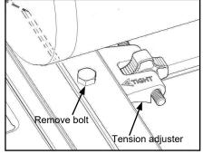
C. Under front bar, loosen tension adjuster bolt, do not remove.
