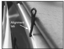
C. Slide left tension adjuster until it engages under side rail (see Step 4F). Push bar back and forth to line up holes. Do not turn adjustment wheel. Insert bolt from top then secure with washer and nut from bottom.
