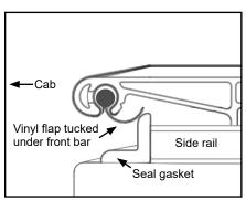
F. With the tension adjuster's support tab under side rail, tighten bolt (left loose earlier) under front bar on each tension adjuster.
