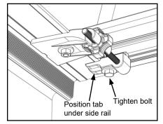
F. With the tension adjuster's support tab under side rail, tighten bolt (left loose earlier) under front bar on each tension adjuster.
