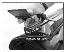
B. Turn 1-1/4" bolt with flat washer onto nut in front bar. Leave loose for now. Repeat for tension adjuster (marked "R") on passenger side of cover and leave bolt loose.
