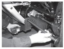
Step 5. Turn ATV wheels to side, and with mount held in place, insert mount pin all the way through.
