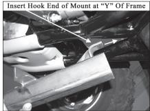
Step 1. Insert hook at rear of mount into "Y" at center of ATV frame and push to engage hook.
