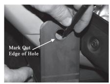
Step 3. With mount held up firmly, use hole to mark for notch cut out of plastic skid plate.
