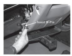
Step 6. With mount pin all the way through opposite side, insert R-pin into small hole of mounting pin.
