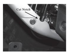
**Step 4.** Using nipper or dremel, cut notch as shown on both sides of skid plate.
