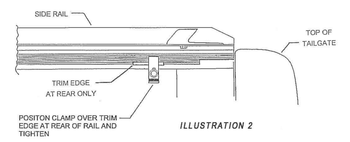
\* NOTE: FOR TRUCKS WITHOUT PLASTIC BED RAIL CAPS, YOU MAY NEED TO REMOVE THE TRIM EDGING FROM THE RAIL BEFORE INSTALLING THE 2 REAR CLAMPS
