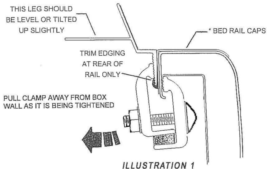
At rear of pickup box, hold rail flush with top of tailgate protector.
