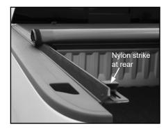
B. Close tailgate slowly, top of tailgate should fit snug under rear bar. If cover impedes normal tailgate operation, raise side rails by: loosening rear clamps, adjusting side rail up and then tightening clamps. If there is a gap between tailgate and cover, adjust side rails lower.
