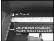
**NOTE:** Before tightening, ensure the vinyl flap is tucked under front bar.
