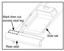
C. Peel paper back, align and adhere seal to end of side rail.
