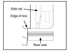
B. Mark seal leg then cut notch in seal.
