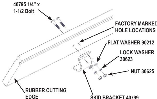
TIP: When mounted - skid bracket should align flush with or slightly above bottom of rubber.
