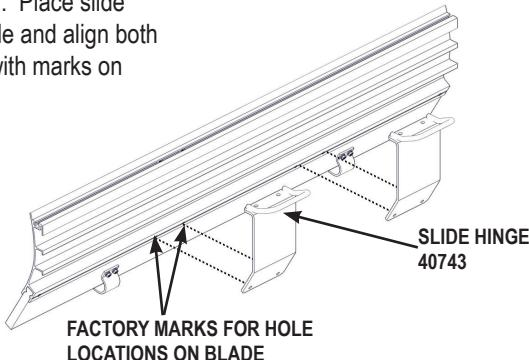
**TIP:** When mounted - slide hinges should measure about 14-1/2"
