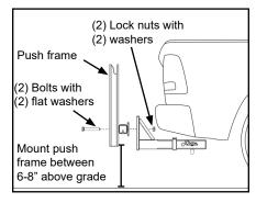
**NOTE**: In some cases, clearance under receiver may be less than 6". If so, plow will still operate properly, but ground clearance will be limited. Use care on uneven surfaces.
