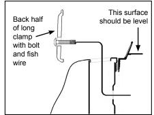
C. Using fish wire, align and pull bolt through hole on inside box wall and hold there for next step.
