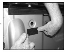
B. At top of rear stake pocket, lower back half of long clamp with fish wire and carriage bolt into pocket.
