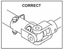
F. Ensure U-joint is in correct position for maximum strength when locked at 90° angle. Make correction if needed.
