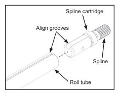
B. Use hole in spline cartridge as guide and measure in 1-5/16" from edge of roll tube. Mark and drill 7/16" hole through first layer of roll tube.
