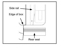
B. Mark seal leg and then cut notch in seal.
