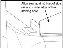
IMPORTANT: Ensure raised portion of seal is against inside edge of box while unraised portion is toward cab.
