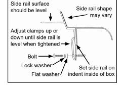
B. At front of box, install first long clamp using a new bolt, lock washer and flat washer. Turn bolt into existing threaded sleeve in box wall.
