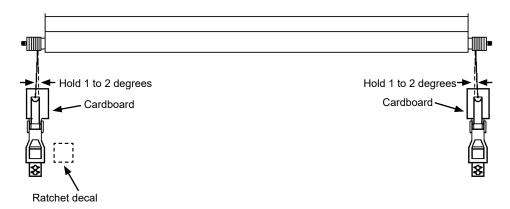
Q. Set cable tension with ratchets. Watch the tension channel on side of spool turn as ratchet applies tension. Proper tension is achieved when tension channel is level at bottom. Once tension is set, remove cardboard.
