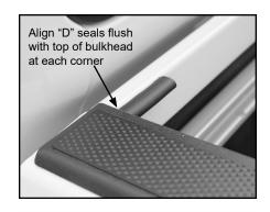
B. Position front of side rail 1/4" away from bulkhead and flush with top of box.
