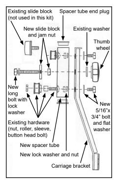
C. Replace both carriage brackets at front of box and slide to rear. Mount bed extender to brackets. Ensure stop block at rear of track is tight to prevent bed extender from sliding too far back. Repeat Steps 2A, 2B and 2C to install side rail on opposite side.
