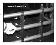
B. Remove carriage bracket by loosening thumb wheel and sliding bracket toward front of box until assembly comes out of track system.
