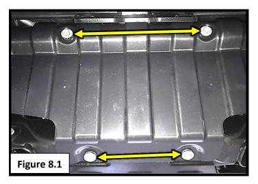
• Remove the factory skid plate and set it aside.
