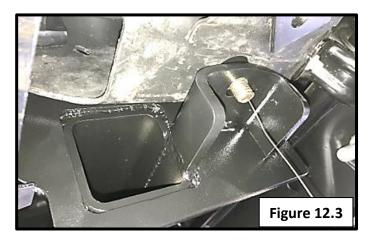
• Secure the 1/2"-13 x 1/3/4" bolt using one 1/2" flat washer, one 1/2" lock washer, and a 1/2" hex nut. See figure 12.4.
