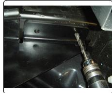
5. Fishwire 1/2-13 x 1 3/4" carriage bolts and SP6 spacers through the access holes and out drilled holes.
