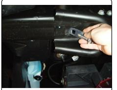
**FISHWIRE TECHNIQUE** NSERT COILED END OF FISHWIRE TOOL THROUGH HITCH MOUNTING HOLE IN VEHICLE FRAME RAIL AND OUT THE ACCESS HOLE. PASS COILED END OF FISHWIRE THROUGH SPACER AND THREAD BOLT INTO COIL. KINK WIRE TO KEEP SPACER SEPERATE FROM BOLT AS SHOWN. PULL FISHWIRE, SPACER, AND BOLT THROUGH FRAME AND OUT MOUNTING HOLE. USE FISHWIRE TO GUIDE HITCH DURING MOUNTING AND PREVENT LOSS OF BOLT / SPACER INSIDE FRAME RAIL. \*\*NOTE: SOME VEHICLES MAY FISHWIRE THROUGH END OF FRAME\*\*
