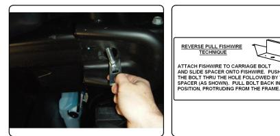
ATTACH FISHWIRE TO CARRIAGE BOLT AND SLIDE SPACER ONTO FISHWIRE. PUSH THE BOLT THRU THE HOLE FOLLOWED BY THE SPACER (AS SHOWN). PULL BOLT BACK INTO
