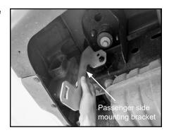
D. Thread second serrated flange bolt into double weld nut through upper hole at top of mounting bracket and round hole in frame. Do not fully tighten.
