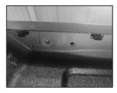
A. On one side at front stake pocket, from underneath box rail drill 3/8" hole through hole closest to cab of stake pocket cover.
