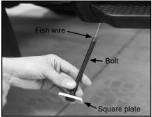
E. Pull fish wire up so bolt is accessible from top, then remove fish wire while holding bolt. Place flat washer and serrated flange nut on bolt, fully tighten.
