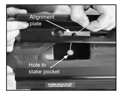
D. Thread bolt with square plate onto fish wire from under truck.
