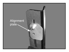
B. Place rack rail on bed rail with alignment plate in rear stake pocket.
