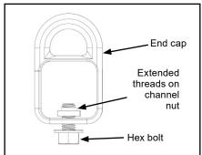
K. Slide channel nut on end cap assembly into cross bar channel. Torque bolt with 9/16" socket to 180 in-lbs (15 ft-lbs).
