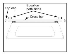
J. Thread 3/8" x 3/4" hex bolt from bottom of end cap bolt hole into channel nut. Leave loose for now.
