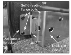
G. Drill 1/4" hole at marked location, then fully secure self-threading flange bolt.
