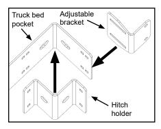
B. Insert (4) carriage bolts, then place (4) nylock flange nuts on bolts. Finger tighten nylock flange nuts on adjustable bracket and fully tighten remaining nylock flange nuts.
