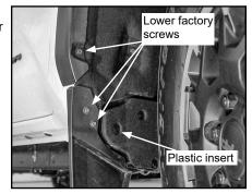
B. Install mud flap with (3) #14 x 1" Phillips head truss screws through 1st, 3rd and 5th slotted holes and 5/16" x 1" hex flange bolt and washer into plastic insert hole into newly free holes in wheel well. Leave hardware loose for now.
