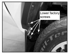
B. Install mud flap with (4) #14 x 1" Phillips head truss screws through 1st, 2nd, 4th and inner slotted holes into newly free holes in wheel well. Leave screws loose for now.
